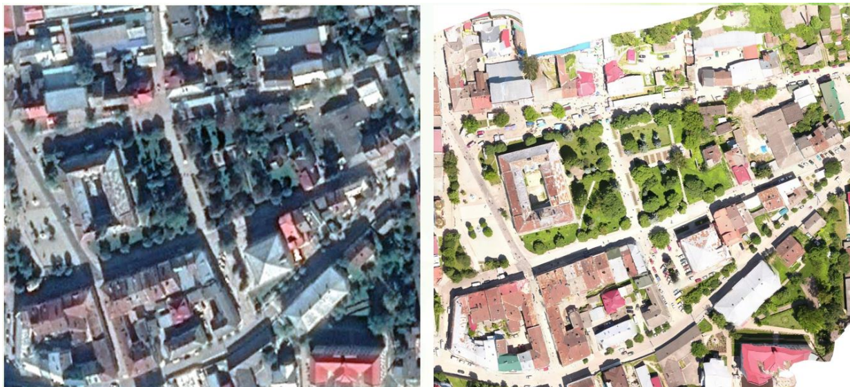
Fig. 1. Comparison of remote sensing materials (on the left) and a UAV orthophotomap of central part of Berezhany town
