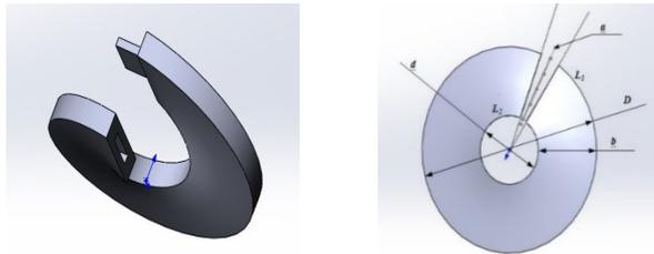
**Fig. 2.** Design scheme of the basic helical element
