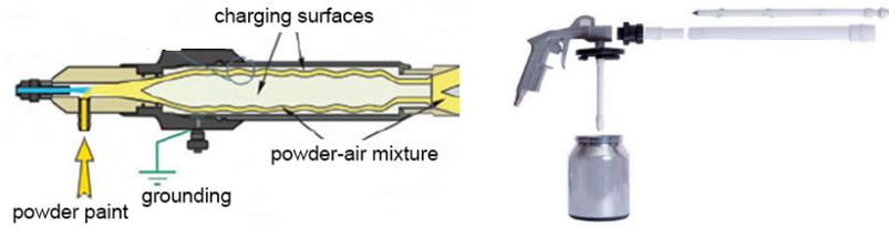
**Fig. 1.** The principle design of the sprayer and the design of the tribo gun
