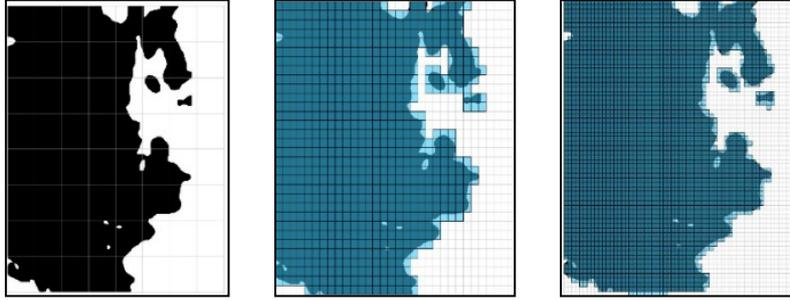
**Fig. 5.** Approximation of the image of the spraying spot by elementary cells with index  $a$
