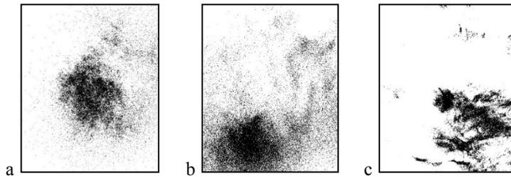
**Fig. 6.** Samples of images of spots spraying powder paints from different manufacturers.
