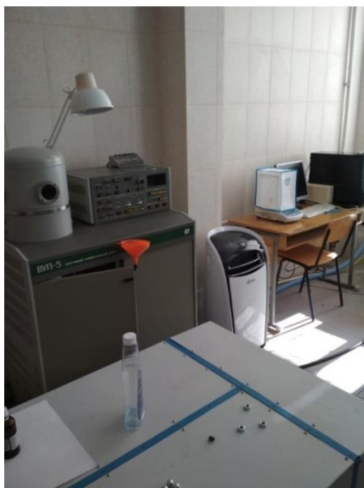
Figure 1 – Vacuum post VUP-5 with a special insert for testing materials for gas emission
