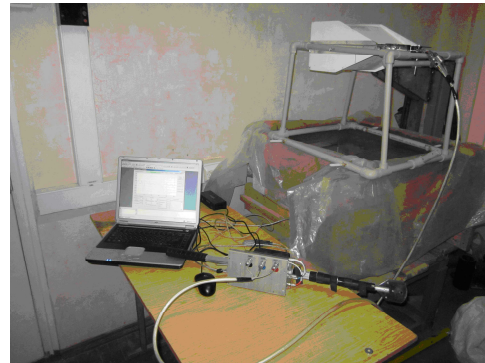
Figure 2. Soil model sounding by georadar complex “ODIAG-1”
