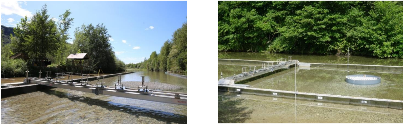
Fig. 2. (a) View of the in-stream flume with a movable floatable platform and array of ADV-velocimeters; (b) Model obstruction of a solid object.
