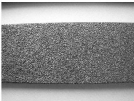
Fig. 4. The appearance of the sample surface, hardened by steel 15H11MFSH
