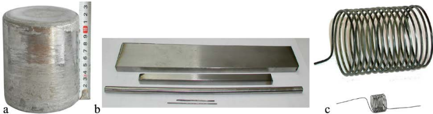
Fig. 2. Ti-55Ni ingot (a) and plates and wire made from it (b, c)
